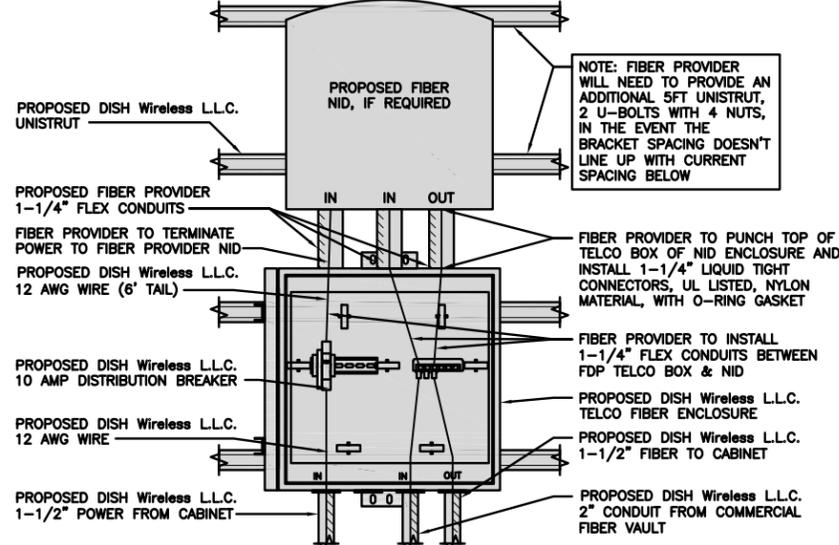
LIT TELCO BOX – INTERIOR WIRING LAYOUT (OPTIONAL)
