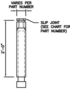
NOTE: CONTRACTOR TO INSTALL EXPANSION FITTING SLIP JOINT AT METER CENTER CONDUIT TERMINATION, AS PER LOCAL UTILITY POLICY, ORDINANCE AND/OR SPECIFIED REQUIREMENT.
