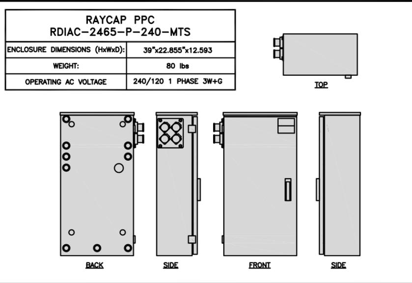
**POWER PROTECTION CABINET (PPC) DETAIL**      NO SCALE      2
