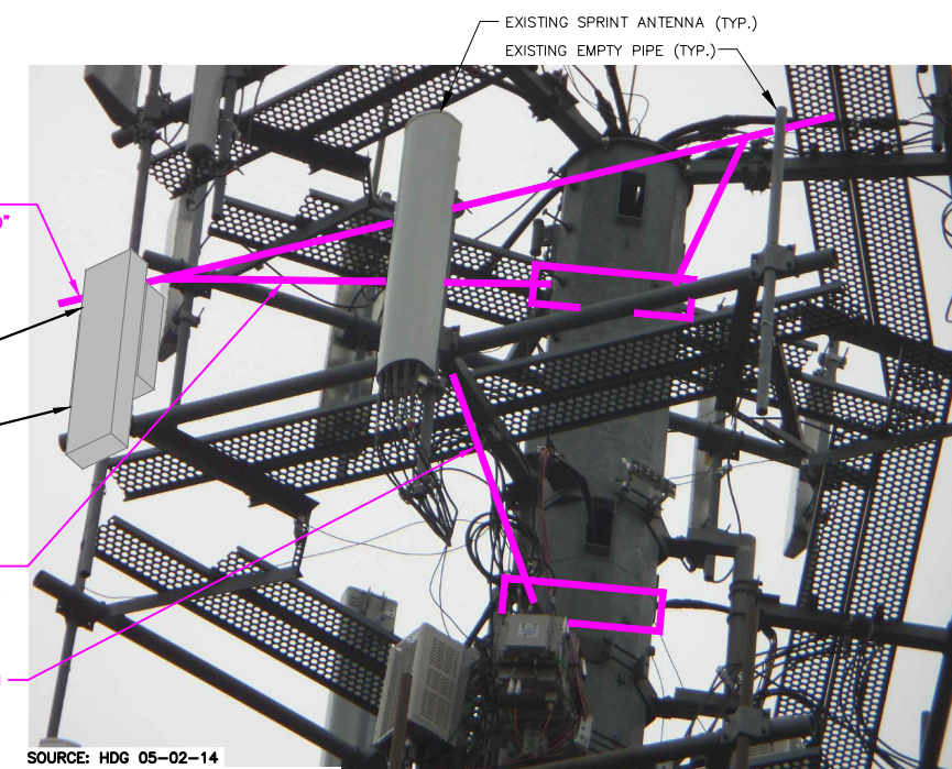
2.5 ANTENNA AND RRH PHOTO DETAIL AND EQUIPMENT SCHEMATIC
