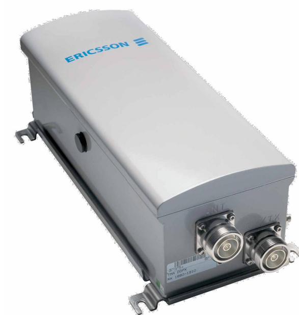
ERICSSON KRY 112 489/2 DIMENSIONS: 11.0"H x 6.1"W x 3.94"D WEIGHT: 15.4 LBS 1 PER SECTOR, TOTAL OF 3
