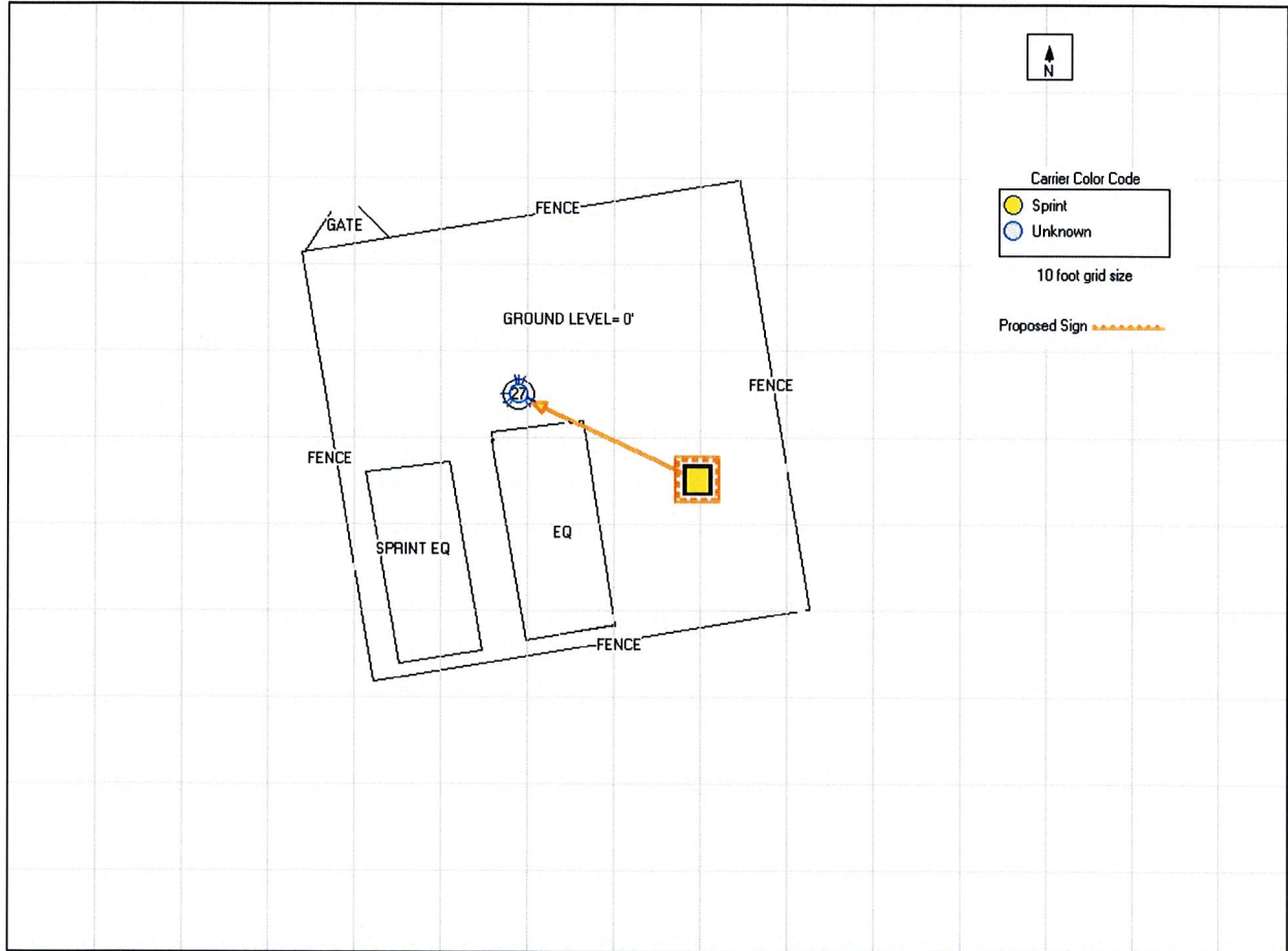
Figure 2: Mitigation Recommendations Caution posted at base of monopole
