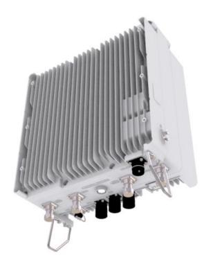
The RFV01U-D2A RU targets dual-band support across Band 13 (700MHz) and Band 5 (850MHz), making it an ideal product for broad coverage footprints across multiple common low-end, long-range frequencies.
