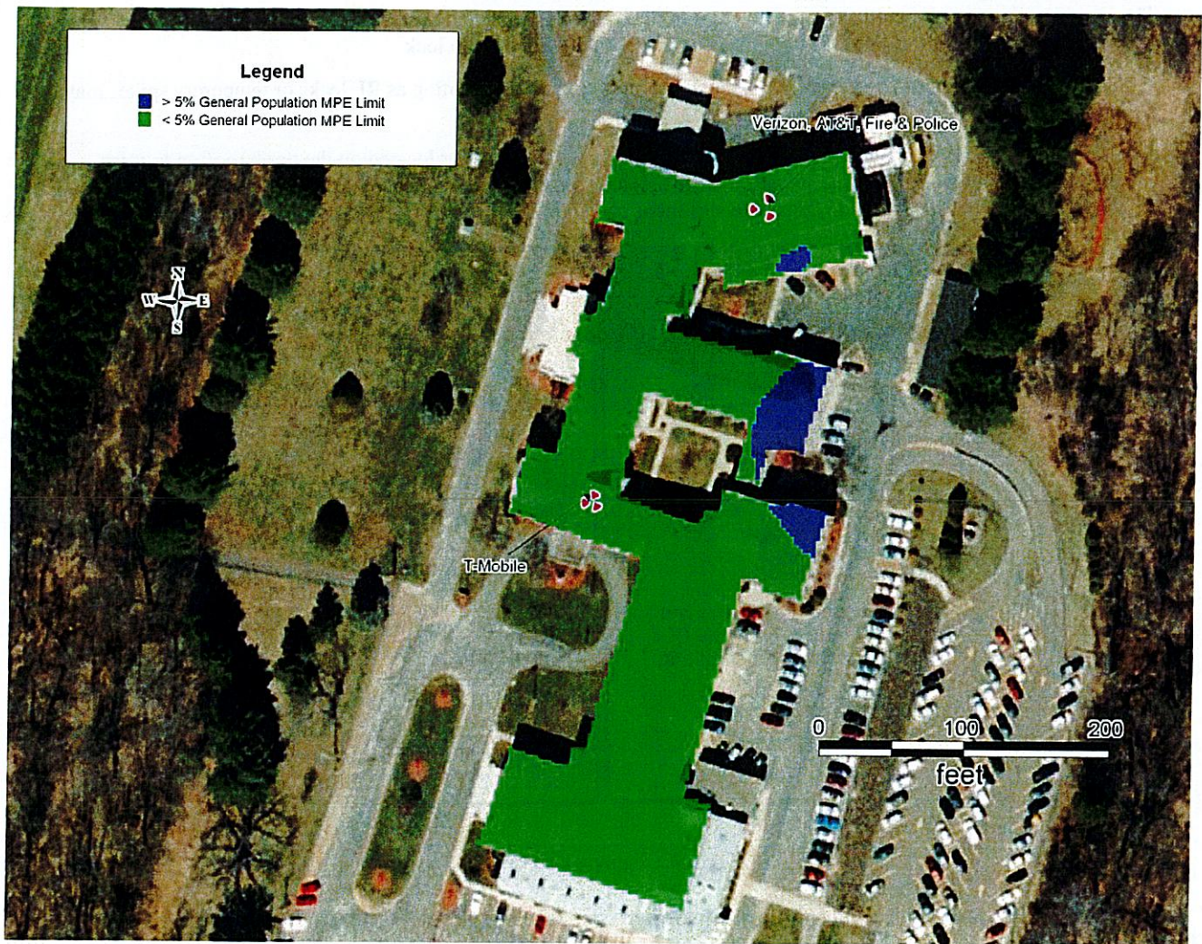
Figure 21: Predicted 5% Levels on Rooftop – Verizon Antennas Only (Post-Modification)
