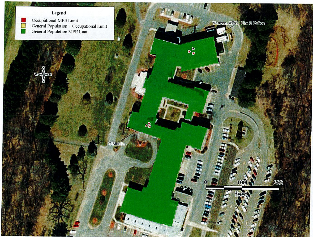
Figure 19: Predicted Power Density Levels on Rooftop – All Carriers (Post-Modification)
