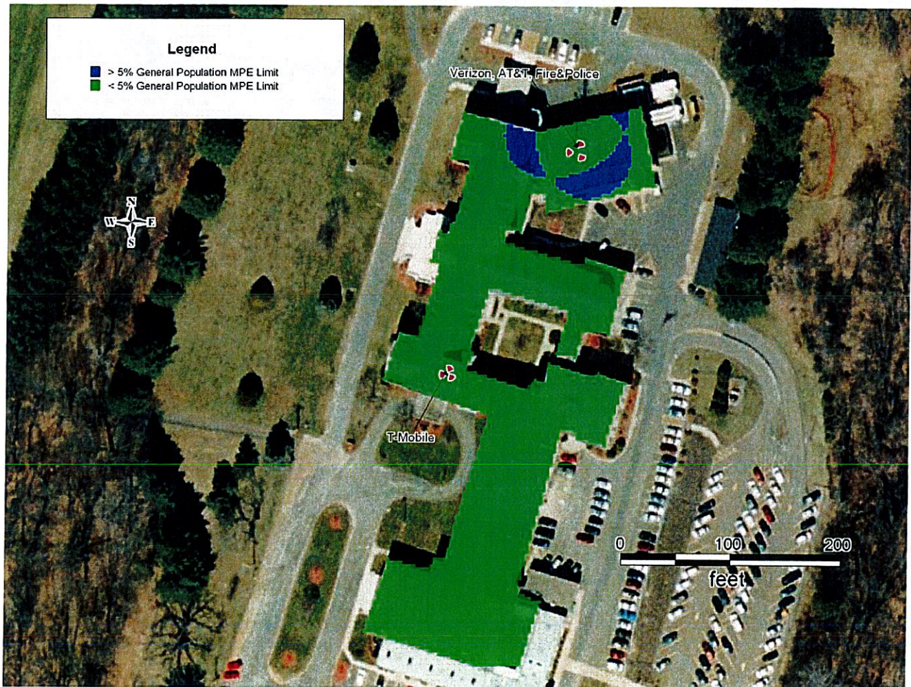
Figure 20: Existing 5% Levels on Rooftop – Verizon Antennas Only
