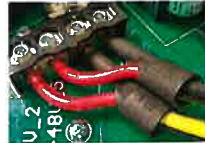
DC Wire Insulator
