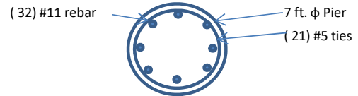
Monopole Pier Foundation
