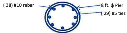
Monopole Pier Foundation
