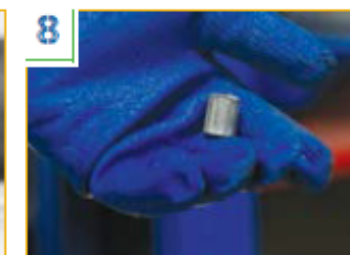
8 Press the small trigger on the shear wrench to eject the bolt spline. The application is now complete.
