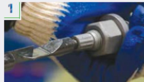
1 Thread the installation tool tip into the splined end of the bolt.
