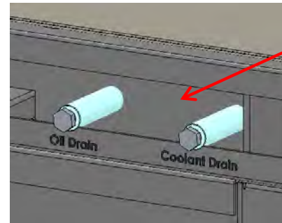
Front Bottom Right Side: External coolant, and oil drains with plugs
