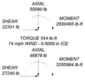
TORQUE 348 lb-ft REACTIONS - 85 mph WIND
