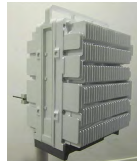
ERICSSON RADIO 4449 B71+B85 DIMENSIONS: 17.9"H x 13.1"W x 10.6"D WEIGHT: 75.0 lbs QUANTITY: 1 PER SECTOR, TOTAL OF 3
