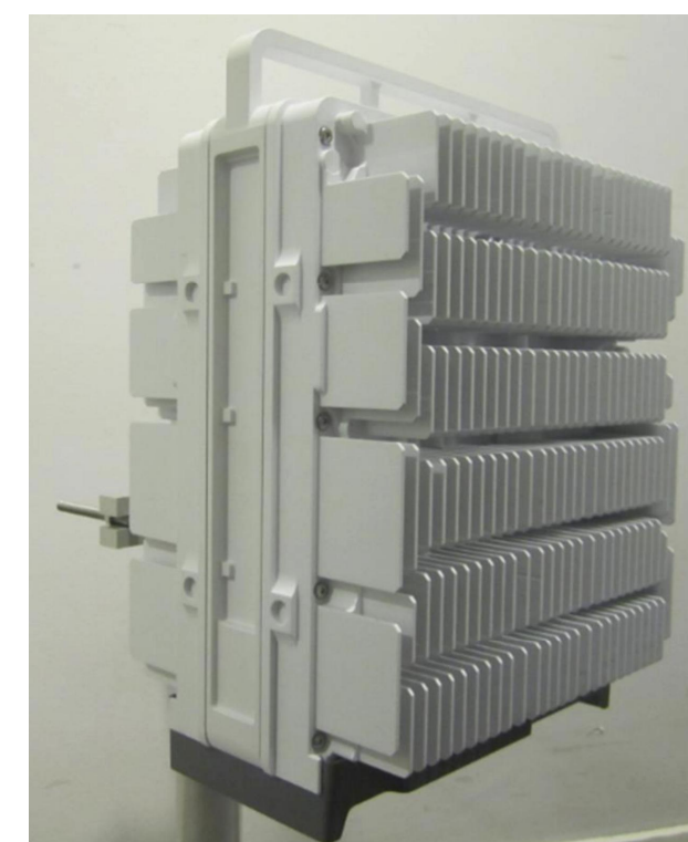
ERICSSON RADIO 4449 B71+B85 DIMENSIONS: 14.9"H x 13.2"W x 9.3"D WEIGHT: 74.0 LBS 1 PER SECTOR, TOTAL OF 3
