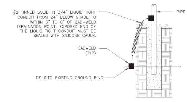
TRANSITIONING GROUND DETAIL SCALE: NOT TO SCALE
