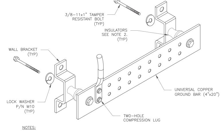
1. DOWN LEAD (HOME RUN) CONDUCTORS ARE NOT TO BE INSTALLED ON CROWN CASTLE USA INC. TOWER, PER THE GROUNDING DOWN CONDUCTOR POLICY QAS-STD-10091. NO MODIFICATION OR DRILLING TO TOWER STEEL IS ALLOWED IN ANY FORM OR FASHION, CAD-WELDING ON THE TOWER AND/OR IN THE AIR ARE NOT PERMITTED.
