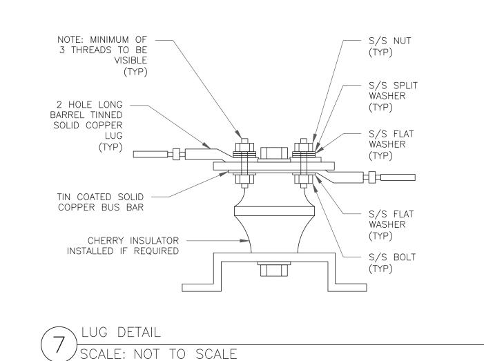
WIRE SIZE BURNDY LUG BOLT SIZE #6 AWG GREEN INSULATED YA6C-2TC38 3/8" - 16 NC S 2 BOLT 3/8" - 16 NC S 2 BOLT #2 AWG SOLID TINNED YA3C-2TC38 #2 AWG STRANDED YA2C-2TC38 3/8" - 16 NC S 2 BOLT 3/8" - 16 NC S 2 BOLT #2/0 AWG STRANDED YA26-2TC38 #4/0 AWG STRANDED YA28-2N 1/2" - 16 NC S 2 BOLT
