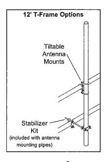
PiRod's 12' Universal T-Frames fit on a variety of different tower types and sizes. Contact PiRod parts department for assistance. (877) GO-PIROD
