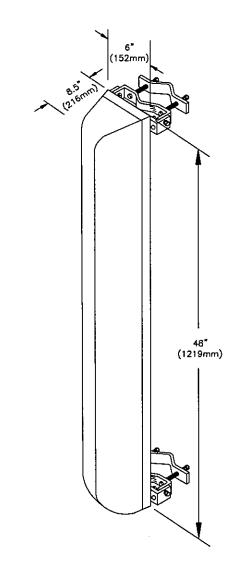
12 dBd (14.1 dBi) Gain Directional Log Periodic Antenna with 90° horizontal 3 dB beamwidth for -SX: 806-896 MHz or -SY: 870-960 MHz.
