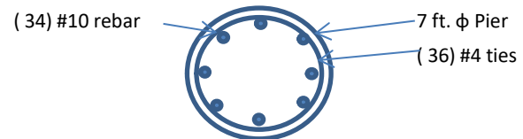
Monopole Pier Foundation
