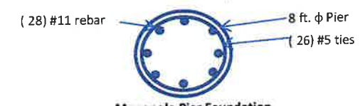
Monopole Pier Foundation
