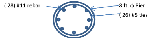
Monopole Pier Foundation
