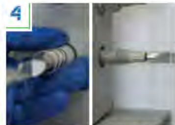
Engage the spring shear sleeve into the shear plane.
