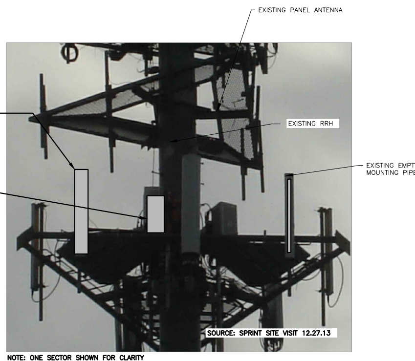
2.5 ANTENNA AND RRH PHOTO DETAIL AND EQUIPMENT SCHEMATIC SCALE: N.T.S.
