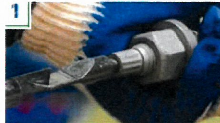
1 Thread the installation tool tip into the splined end of the bolt.
