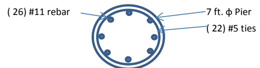
Monopole Pier Foundation
