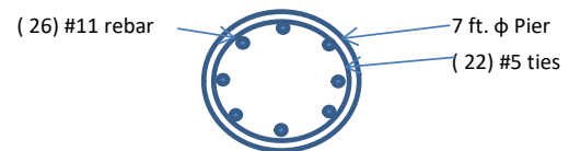
Monopole Pier Foundation
