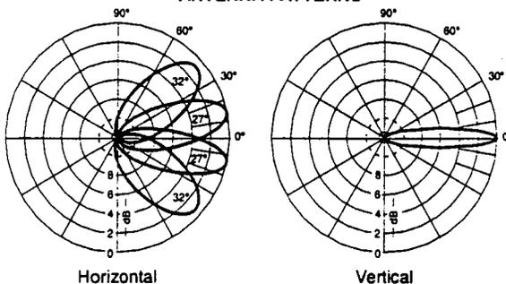
In CDMA systems, SpotLight 2000 combines beams to create custom sector patterns. You can use SpotLight's Beam Controller software to define, model and display CDMA sectors.
