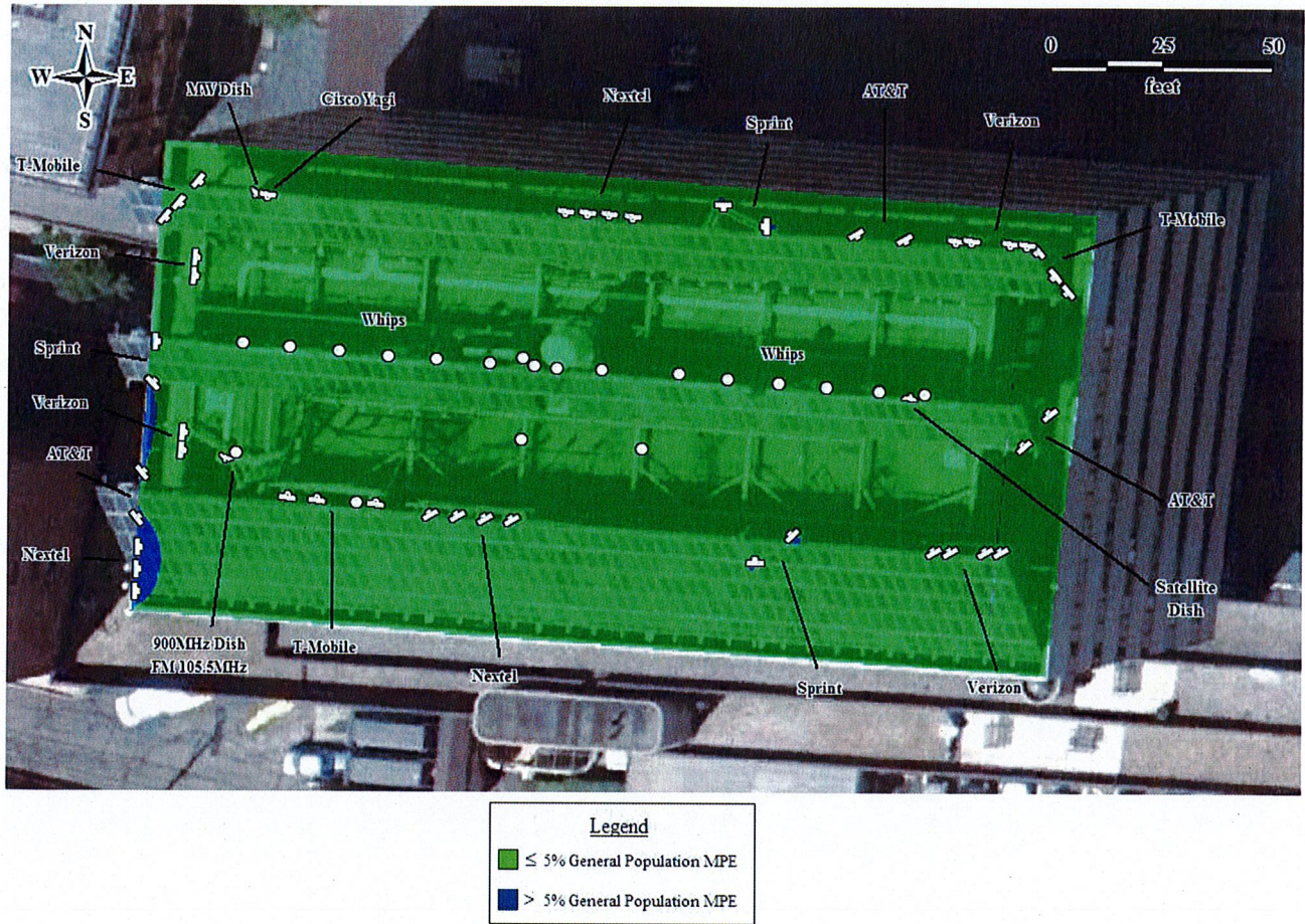
Figure 27: Predicted 5% Levels on Rooftop – Sprint-Nextel Antennas Only (Post-Modification)
