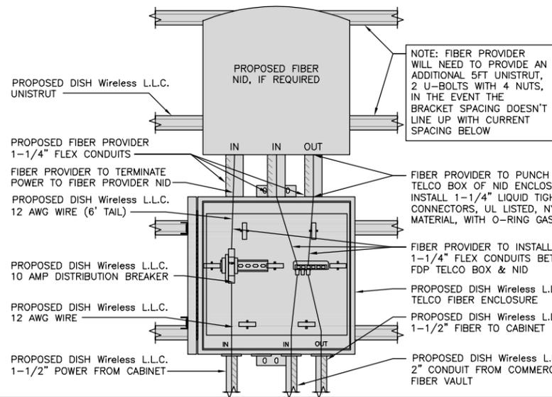
NOTE: FIBER PROVIDER WILL NEED TO PROVIDE AN ADDITIONAL 5FT UNISTRUT, 2 U-BOLTS WITH 4 NUTS, IN THE EVENT THE BRACKET SPACING DOESN'T LINE UP WITH CURRENT SPACING BELOW
