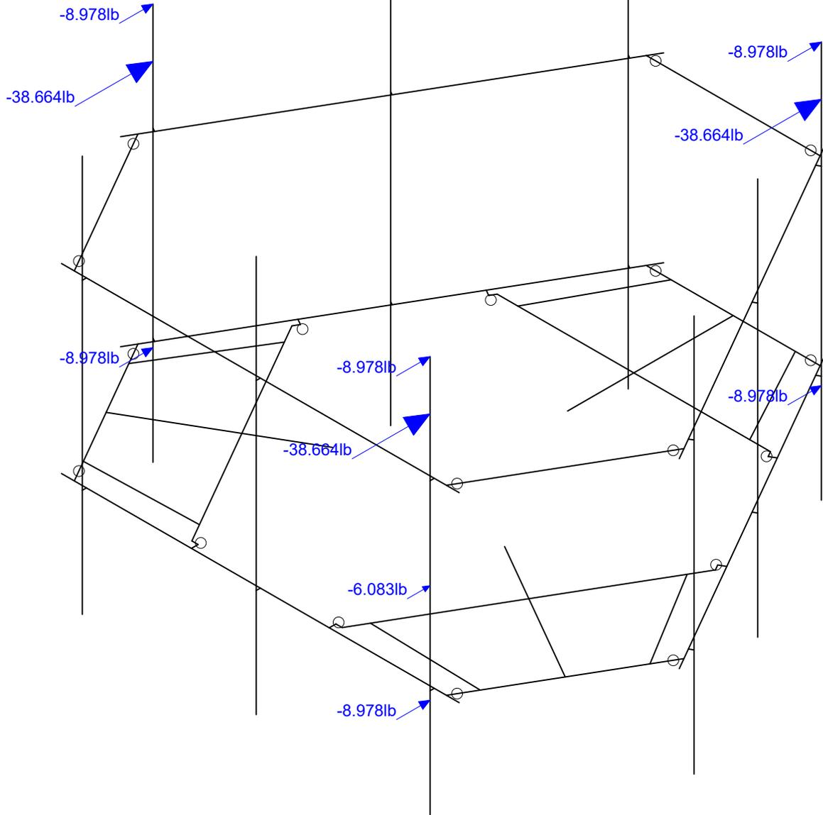
Loads: BLC 31, Seismic Load Z
