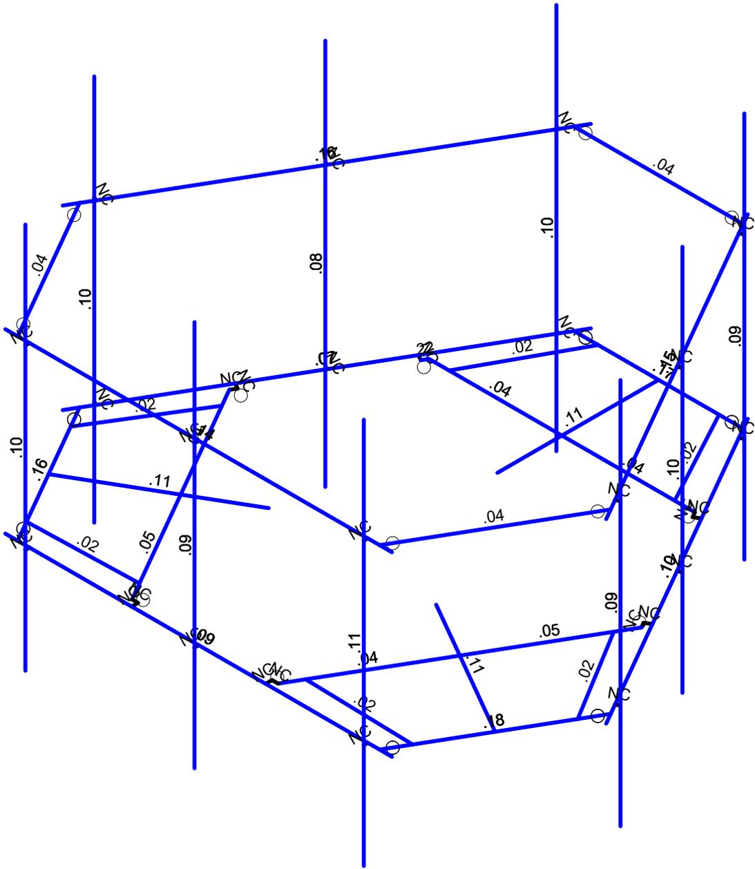
Member Shear Checks Displayed (Enveloped)
