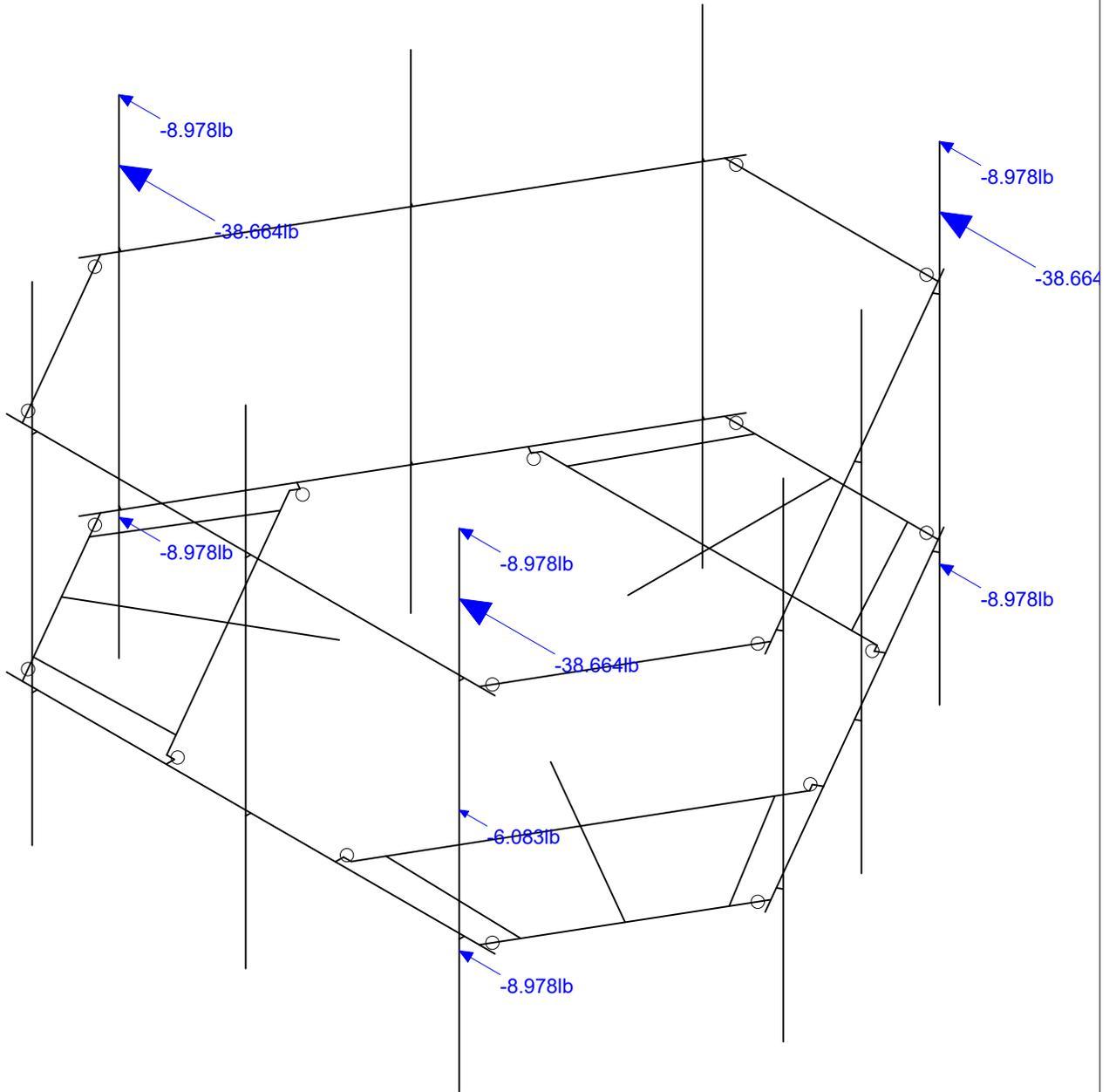
Loads: BLC 32, Seismic Load X
