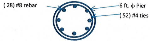
SST Pier Foundation
