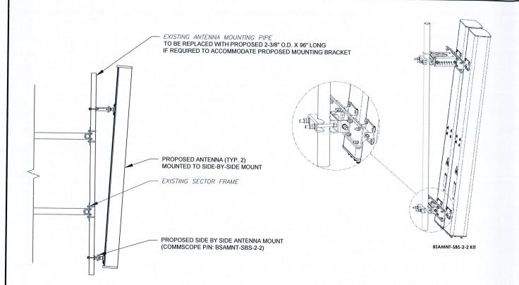
EXISTING MOUNTING PIPE PROPOSED OVP (MOUNT PER MANUFACTURER'S SPECS) (ENSURE THAT BRACKET DOES NOT CONFLICT WITH EXISTING OR PROPOSED EQUIPMENT)
