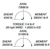
TORQUE 1064 lb-ft REACTIONS - 80 mph WIND
