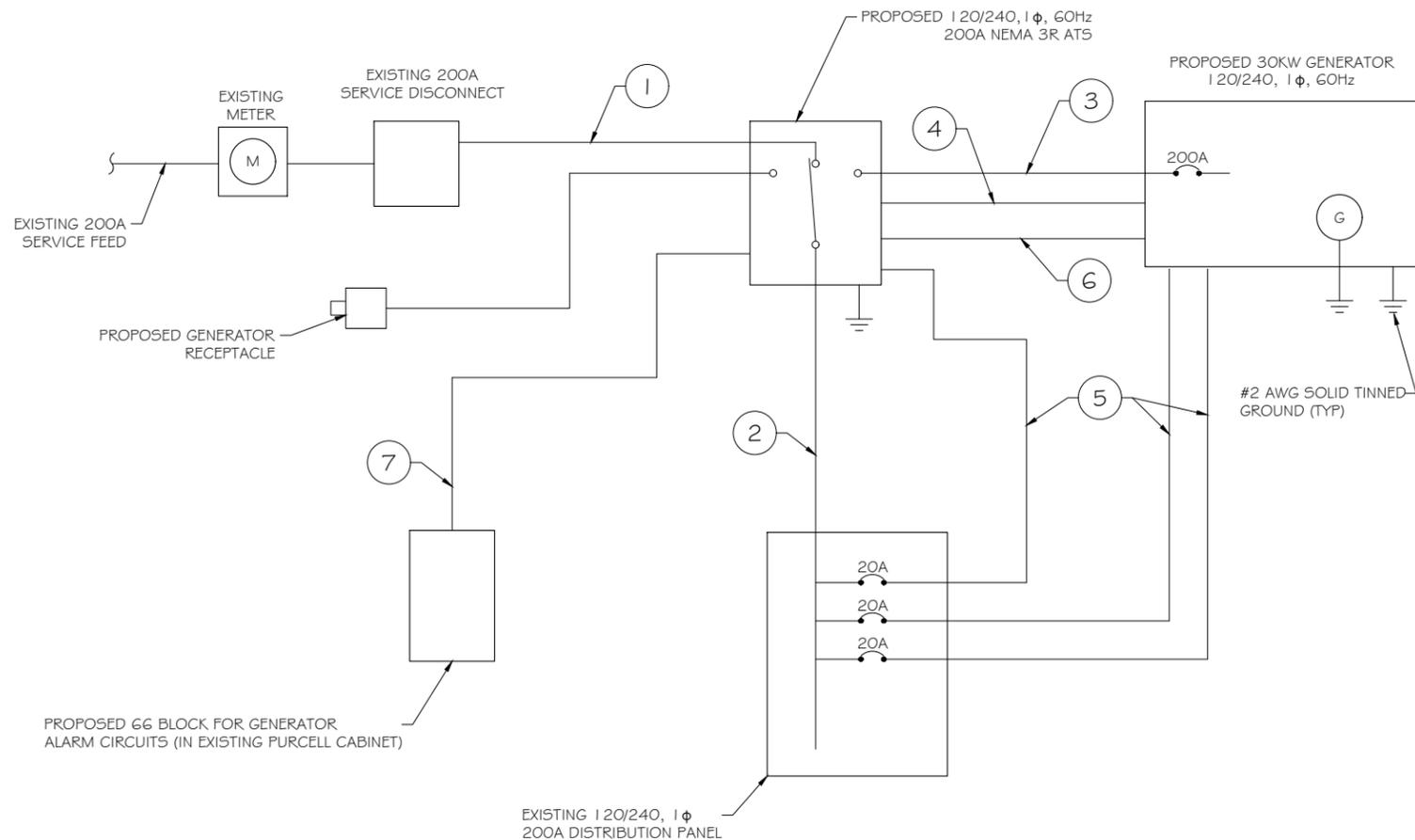
PROPOSED WIRING DIAGRAM
