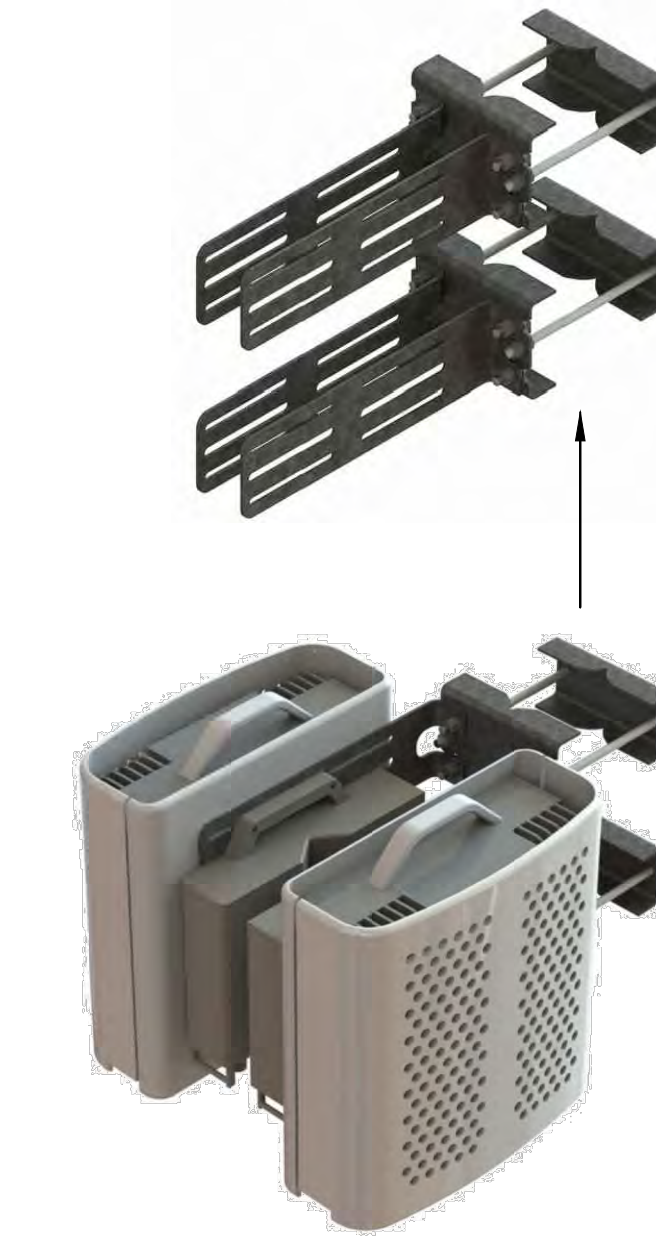
COMMSCOPE RR-FA2 FAST ACCESS DUAL RRU MOUNT KIT DIMENSIONS: 16.4"H x 8.6"W x 18"L WEIGHT: 36.0 lbs QUANTITY: 1 PER SECTOR, TOTAL OF 3
