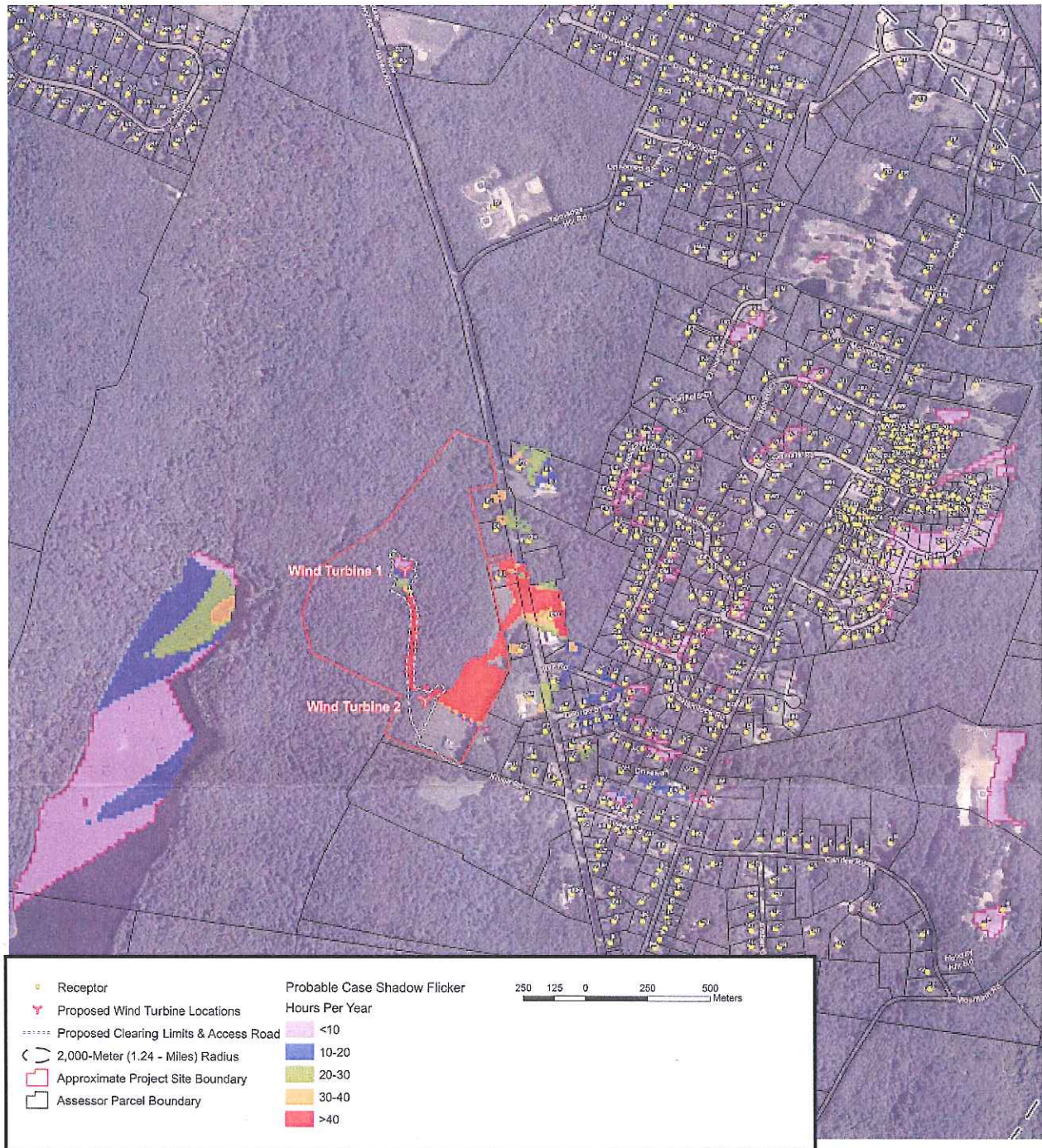
Figure 7: Shadow Flicker Probable Case Model using turbines in original locations with 82.5-meter rotor diameter - showing exterior shadow flicker. Please note, not all areas with <10 hours are shown. Turbine 1 is original northern location. Turbine 2 is southern location. (BNE 2a)
