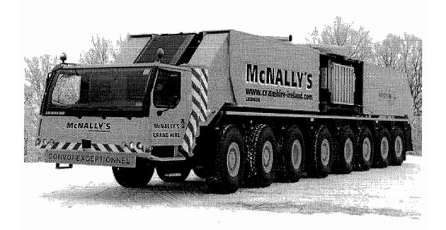
The new crane travelled form the manufacturers Ehingen plant this week directly to its first contract in France where it will be used to erect a number of wind turbines. The unit comes with a maximum system height of 191 metres and is rated at seven metres radius.
