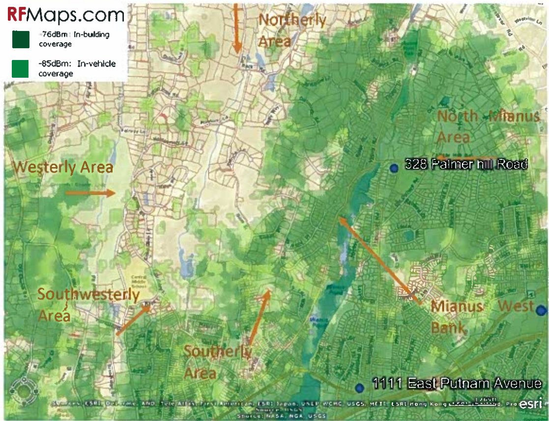
Figure 8 - Coverage Available from Existing T-Mobile Facilities plus the 328 Palmer Site at 35 Feet above Ground.
