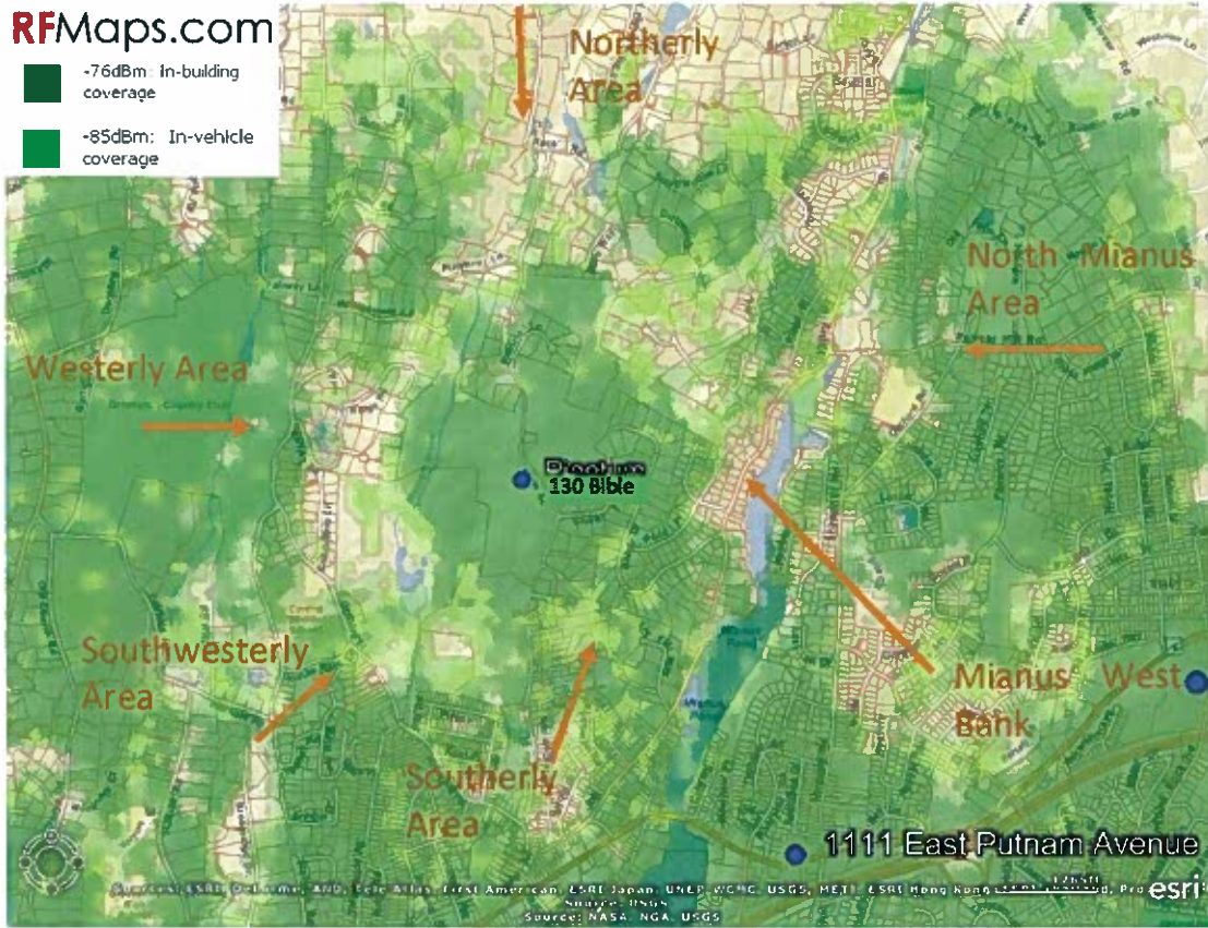
Figure 14- Coverage Available from Existing T-Mobile Facilities plus 130 Bible St Site at 80 Feet above Ground
