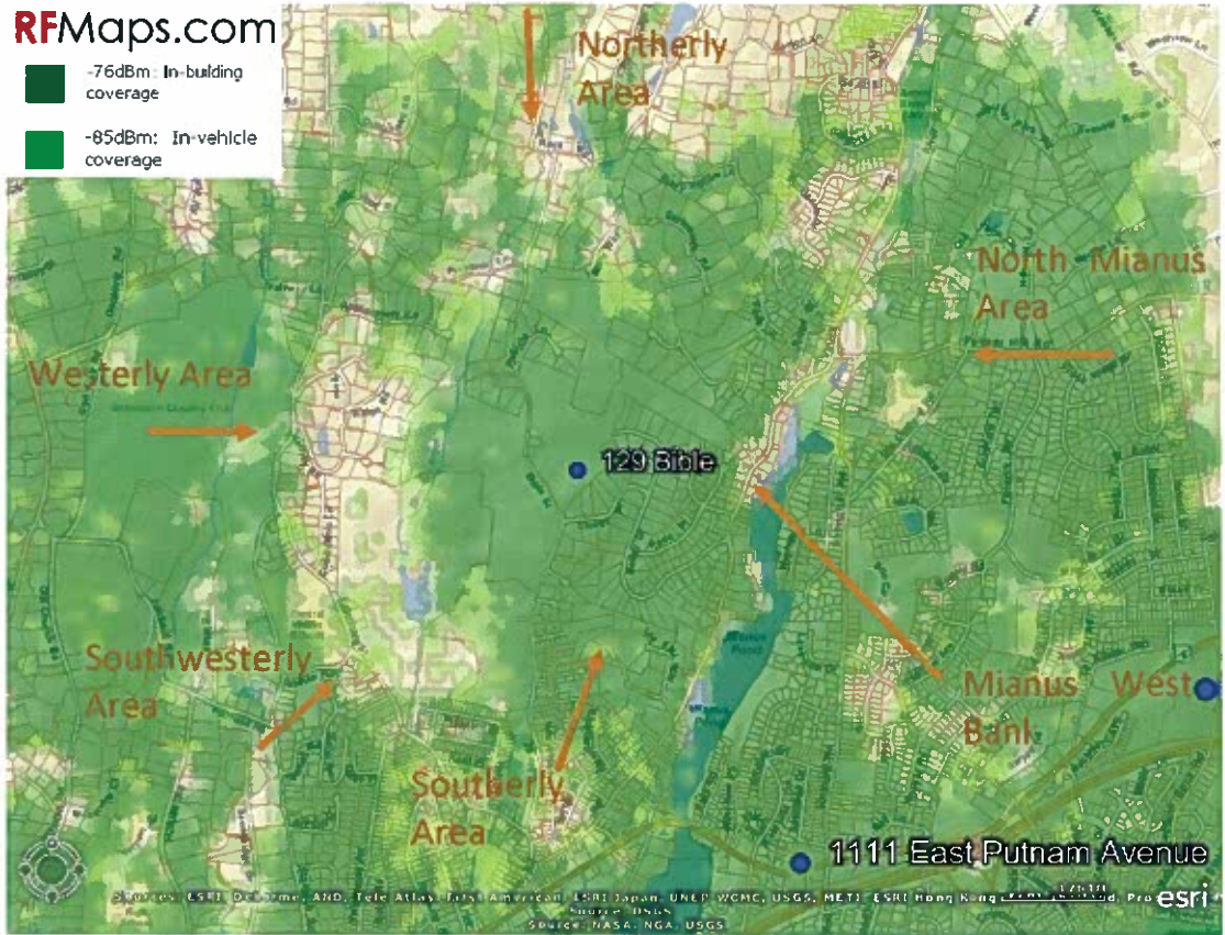
Figure 11 - Coverage Available from Existing T-Mobile Facilities plus the 129 Bible St Site at 80 Feet above Ground
