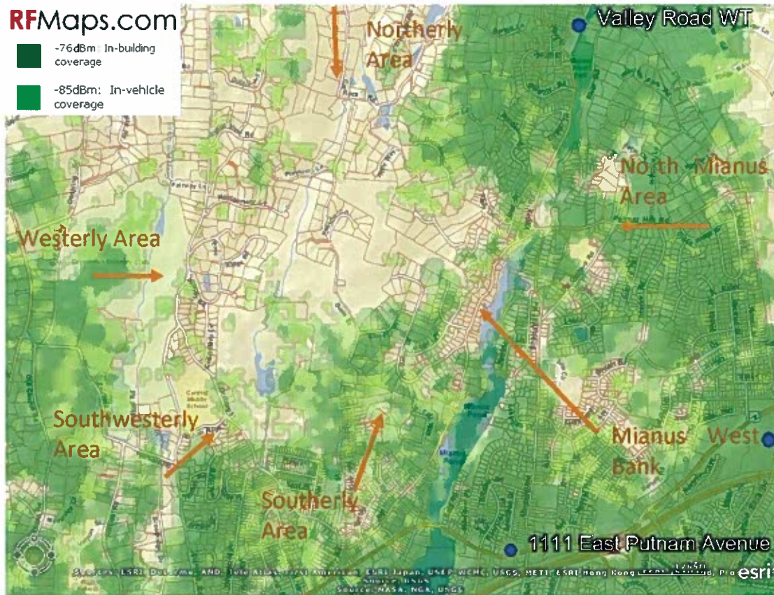
Figure 18 - Coverage Available from Existing T-Mobile Facilities plus Water Tank 50 Feet above Ground
