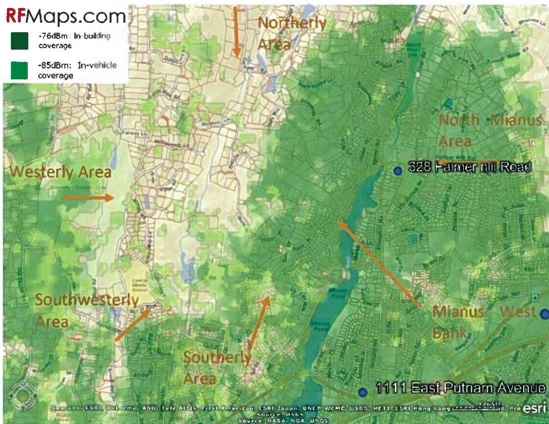
Figure 7 - Coverage Available from Existing T-Mobile Facilities plus the 328 Palmer Site at 80 Feet above Ground.
