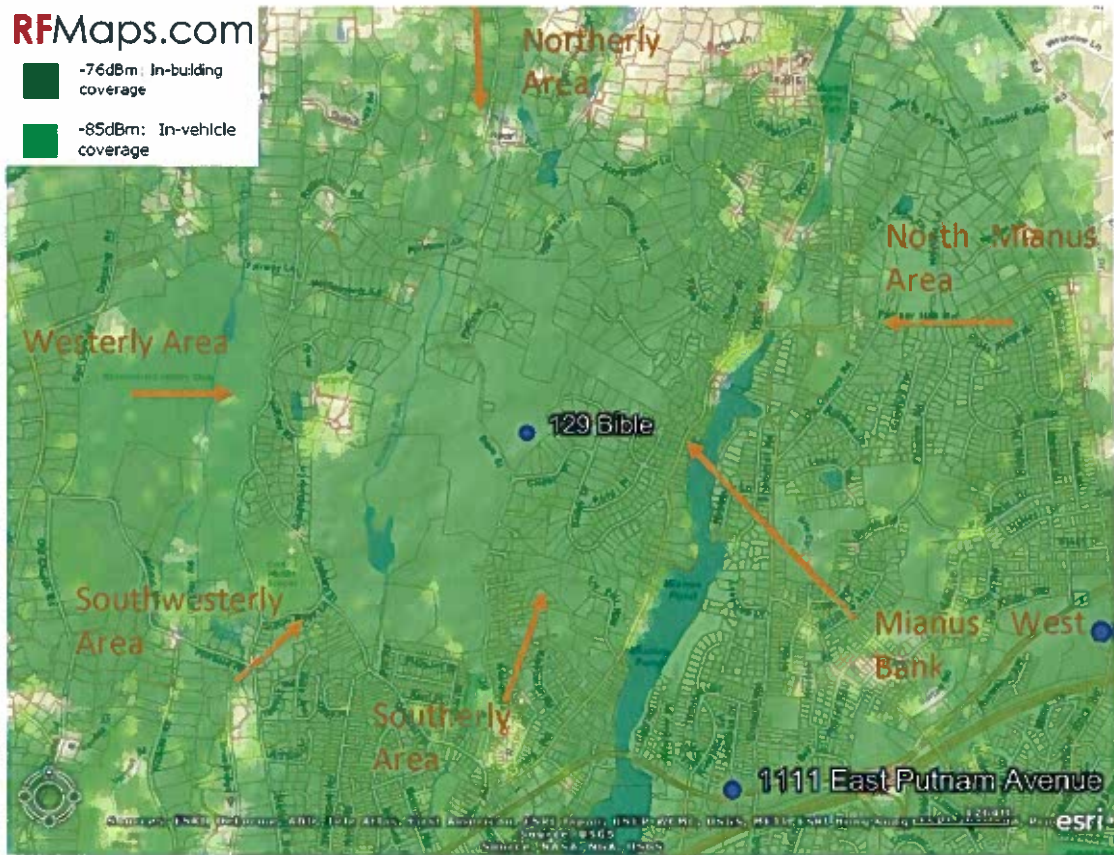
Figure 9 - Coverage Available from Existing T-Mobile Facilities plus the 129 Bible St Site at 160 Feet above Ground.
