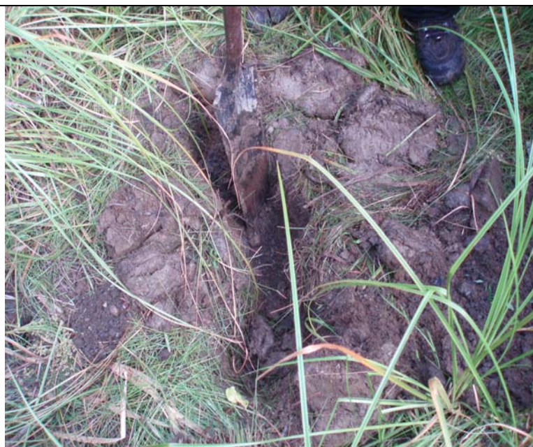
Soil testing in small wetland identified asphalt at a depth of 4-12 inches, resulting in the creation of a perched wetland.
