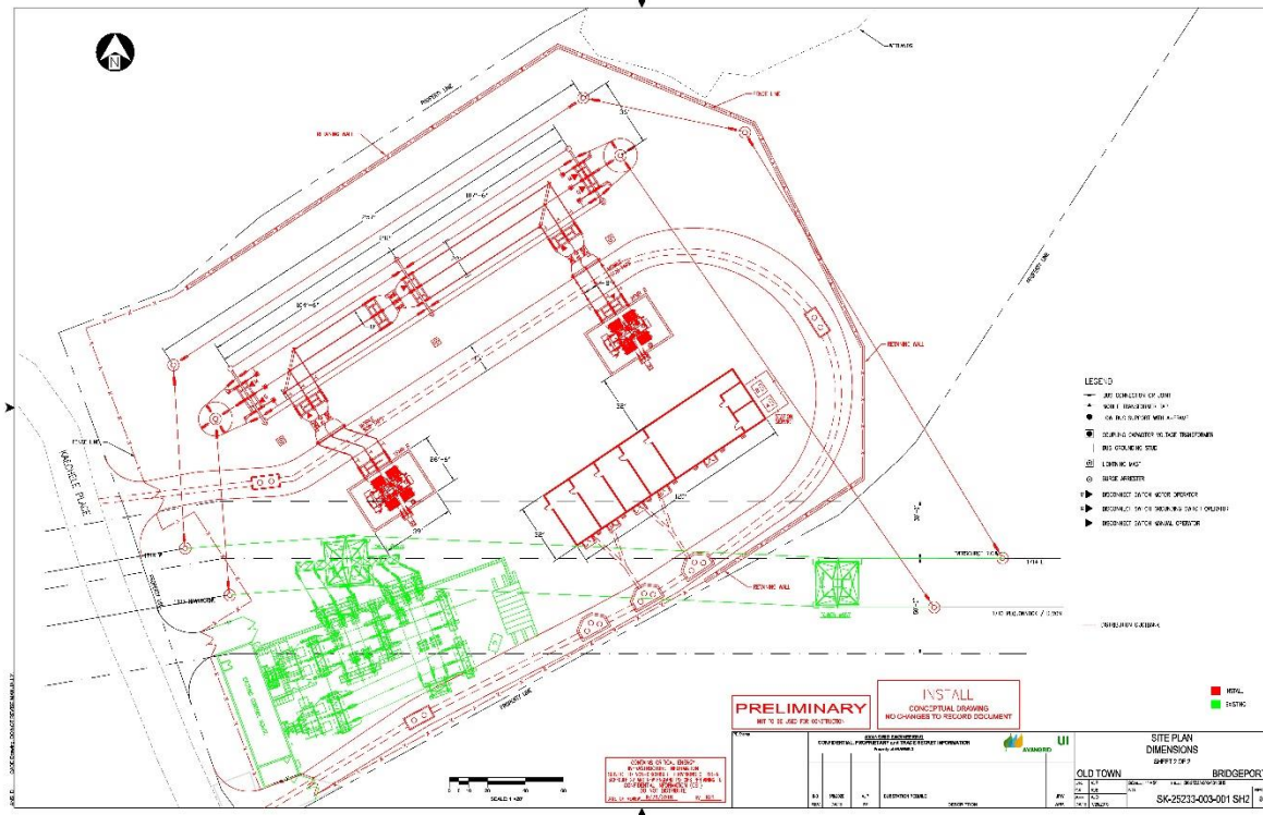
Figure 2-1: Proposed Substation Layout
