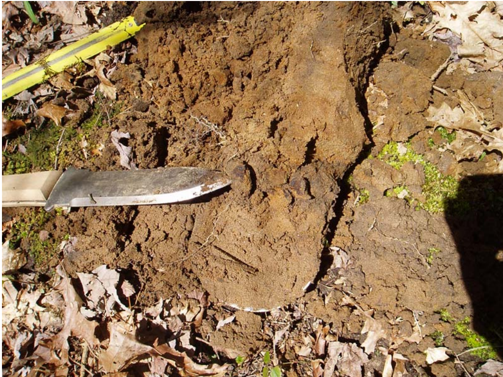
Photo 3: T3-7B (note: knife points to large Fe/Mn nodules/concretions)
