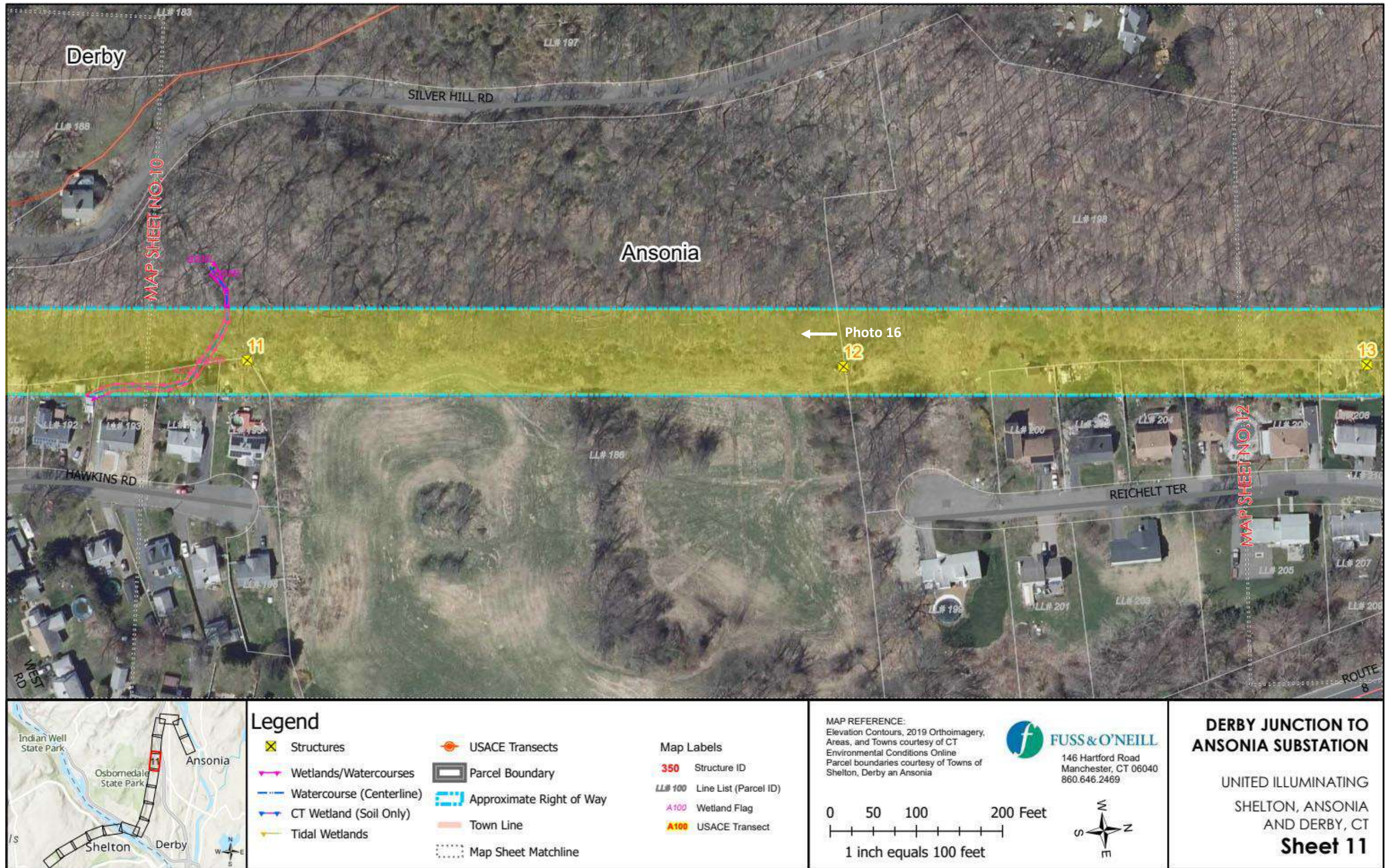
Figure 10; Sheet 11. Project plans showing No/Low and Moderate/High sensitivity areas along the ROW.
