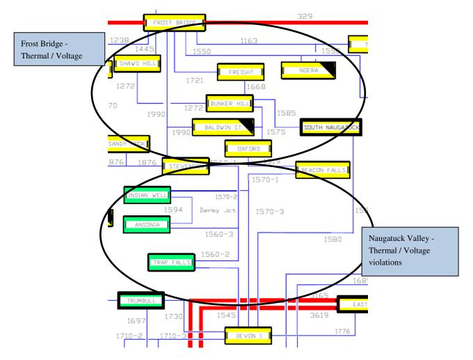
Figure 5-6: Frost Bridge – Naugatuck Valley Thermal and Voltage Violations
