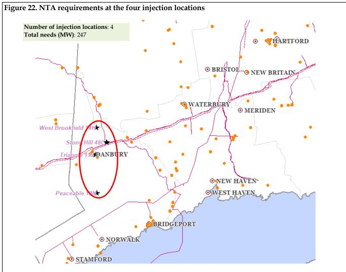
The closest (large) cities are demarcated with red dots; orange dots represent existing generation assets; injection locations are labeled with a blue marker; and gas pipelines are represented by pink lines.
