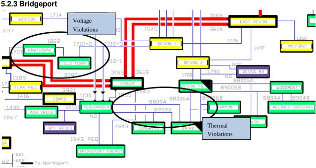
Figure 5-17: Bridgeport Thermal and Voltage Violations
