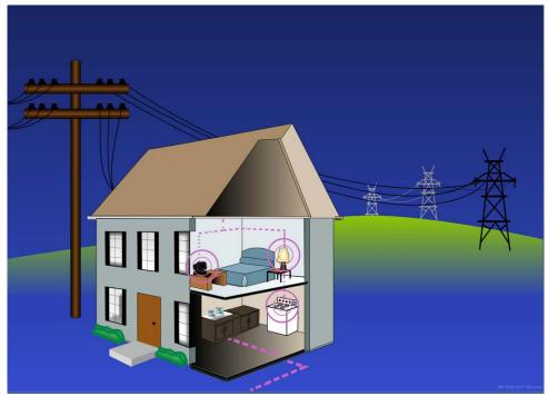
Figure 1. Common sources of ELF EMF in the home (appliances, wiring, currents running on water pipes, and nearby distribution and transmission lines).
