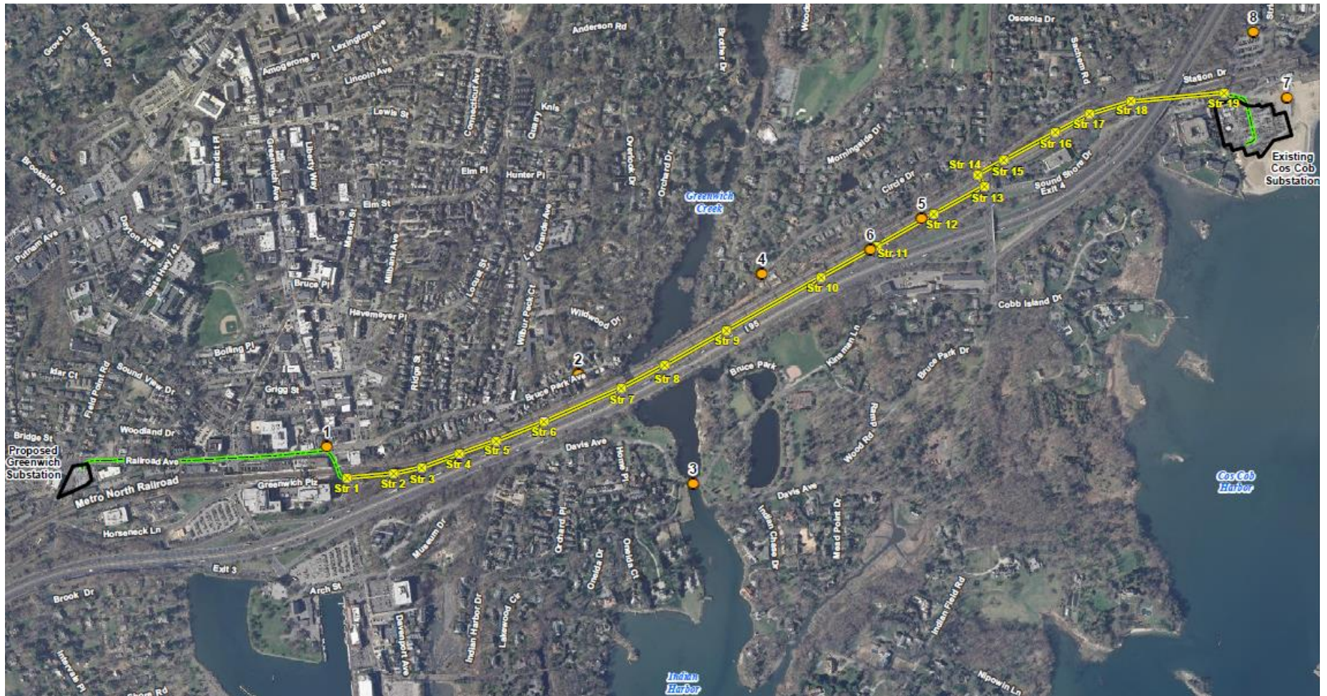
Green denotes underground cable section, yellow denotes overhead line section. - potential structure locations are round yellow dots. (Eversource 44, LF-025)
