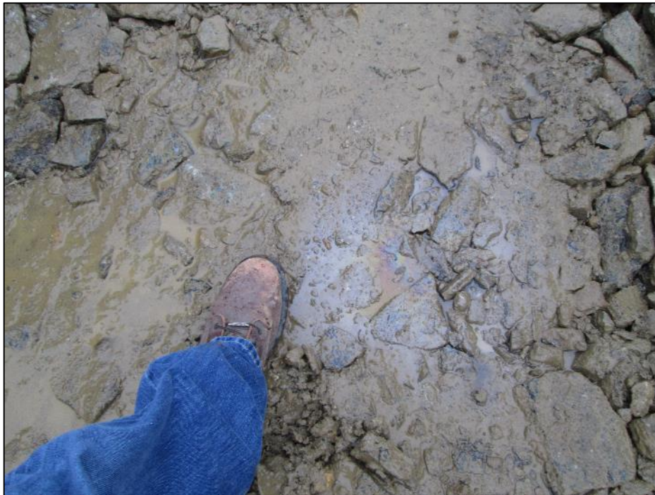
Photo #7: Observed multiple petroleum drips on access road and Str pad 290. (12/3)
