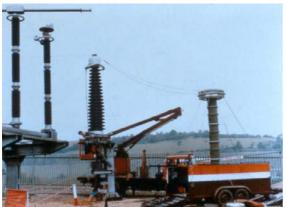
High voltage test set connected to SCFF terminal
