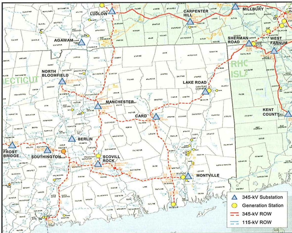
Figure 1-1: Key substations in southern New England.
