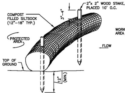
1. SILT SOCK SHALL BE FILTREXX SILT SOCK, OR APPROVED EQUAL.
