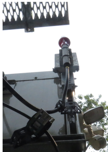
GPS installed with manufacturer supplied hardware
