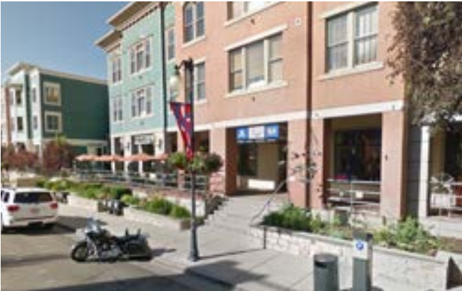
Elevated Storefront with Combination of Platform and Retaining Walls
