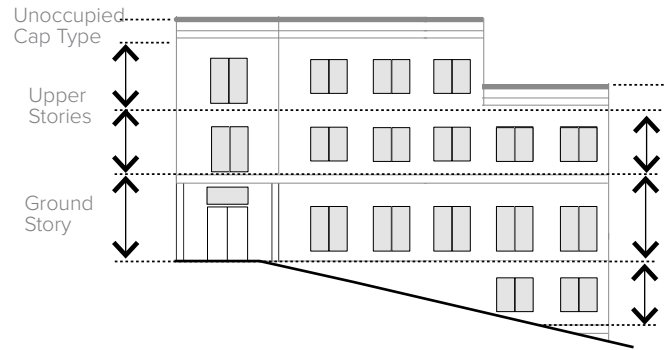
Figure 14-F. Measuring Height along a Sloped Street
