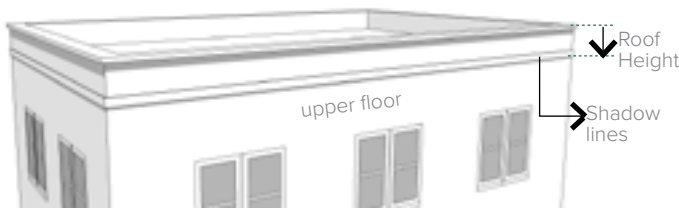
Figure 6-A. Example of a Parapet Roof Type
