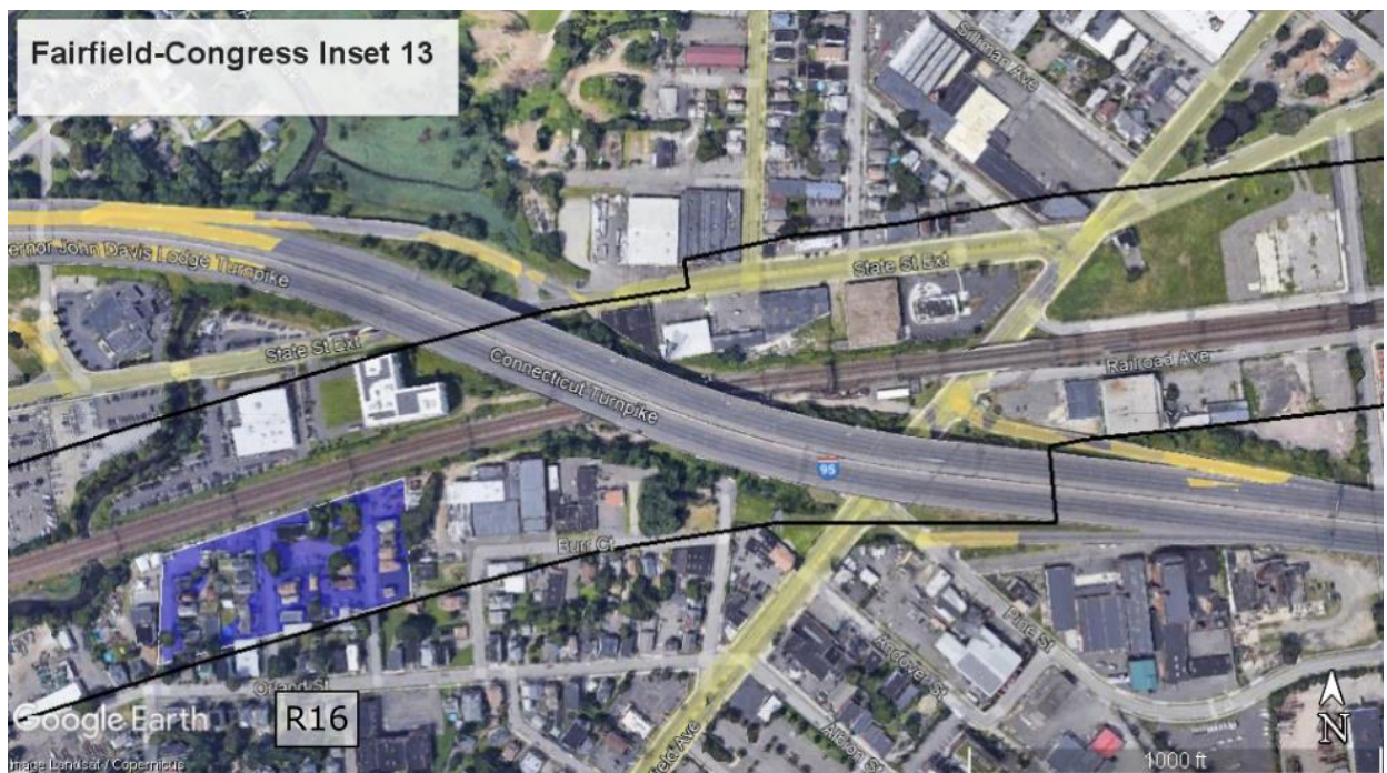
Figure D-14. Measurement areas along the transmission lines. Black lines show the distance of 300 feet from the proposed transmission line. Blue areas are residential, and yellow areas are community facilities.
