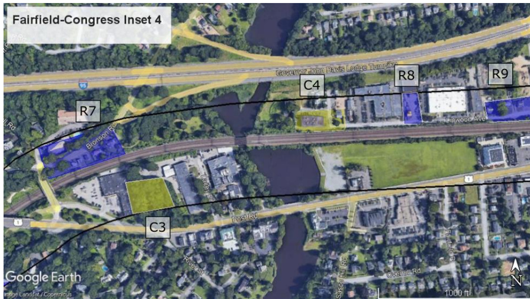
Figure D-5. Measurement areas along the transmission lines. Black lines show the distance of 300 feet from the proposed transmission line. Blue areas are residential, and yellow areas are community facilities.
