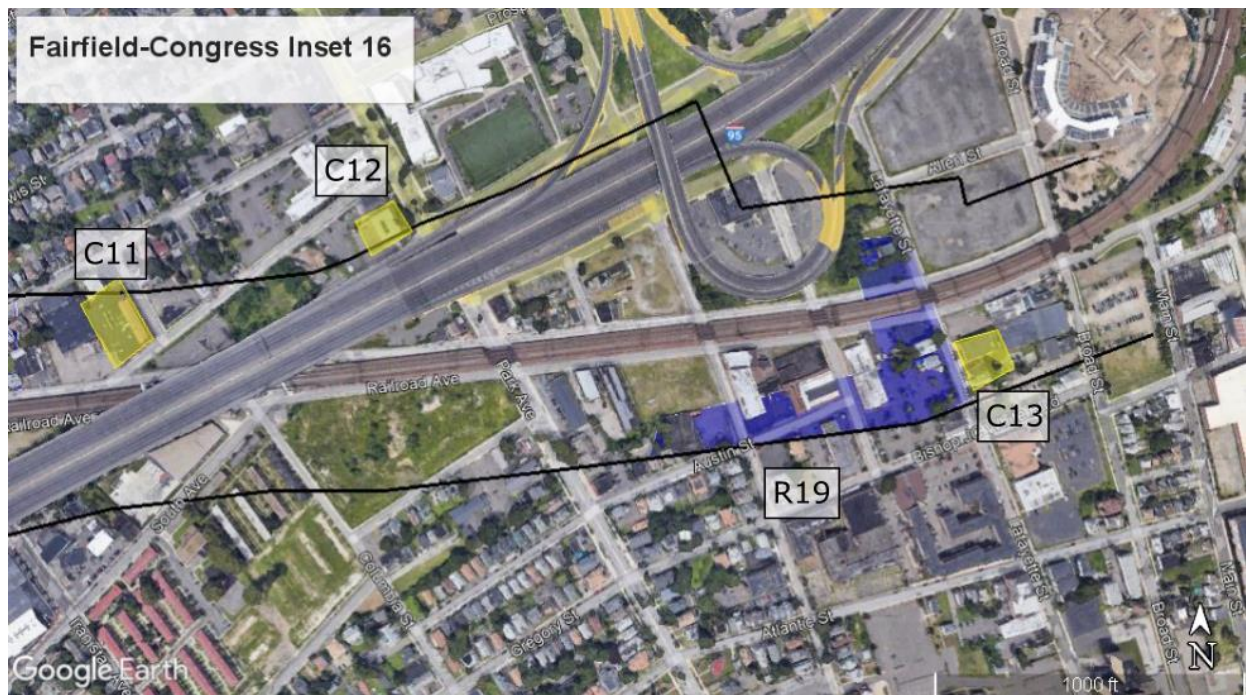
Figure D-17. Measurement areas along the transmission lines. Black lines show the distance of 300 feet from the proposed transmission line. Blue areas are residential, and yellow areas are community facilities.
