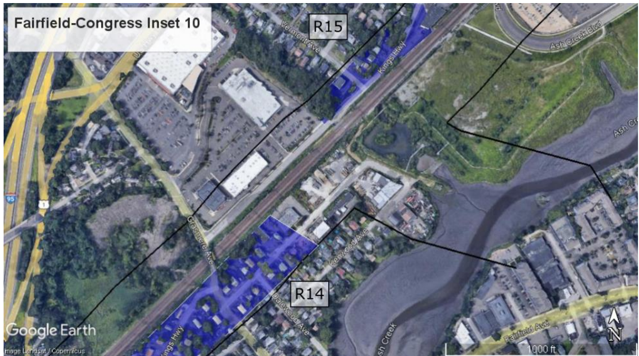
Figure D-11. Measurement areas along the transmission lines. Black lines show the distance of 300 feet from the proposed transmission line. Blue areas are residential, and yellow areas are community facilities.
