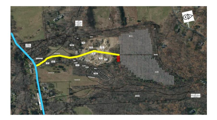
Figure 1. Proposed Site Plan for the 3.5-MW solar photovoltaic generator system in Burlington, Connecticut.
